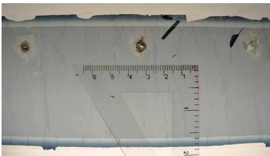
Figure 2. Photograph of an unwound metallized film capacitor having poor self-clearing behavior with damage involving adjacent layers.
