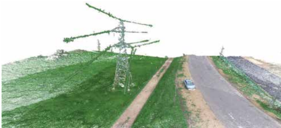
Figure 15. Results of 3D reconstruction of electrical infrastructure.
