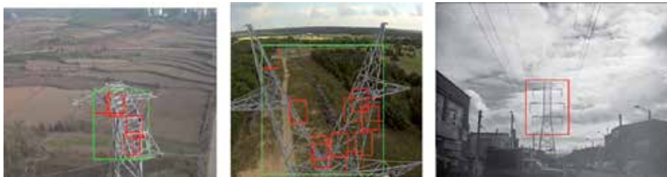
Figure 11. Tower detection examples using SVM and a grid of descriptors.
