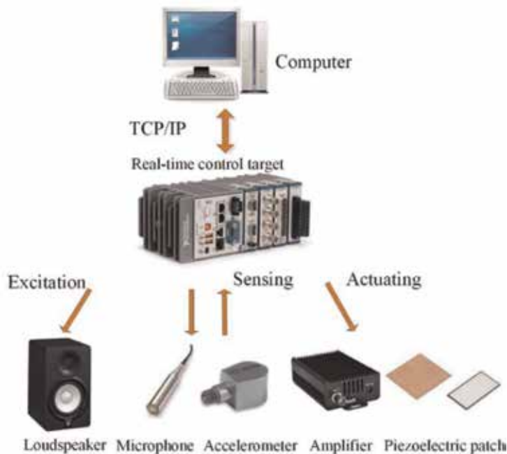
Figure 10. Components of the control system.
