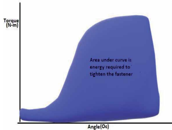
Figure 2. Total energy area required to tighten the bolt fastener.
