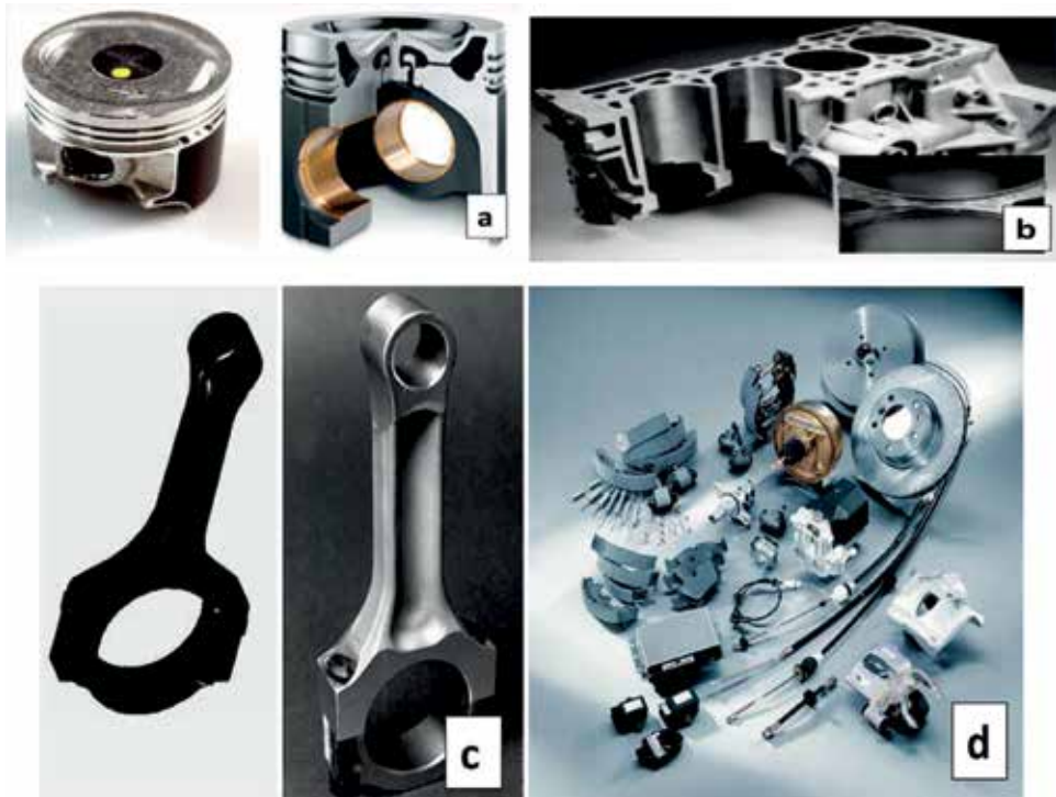
Figure 1. (a) Piston, (b) engine with cylinder barrel, (c) piston connecting rod, (d) brake system made of aluminium (Al) metal matrix composites (MMCs) [13].
