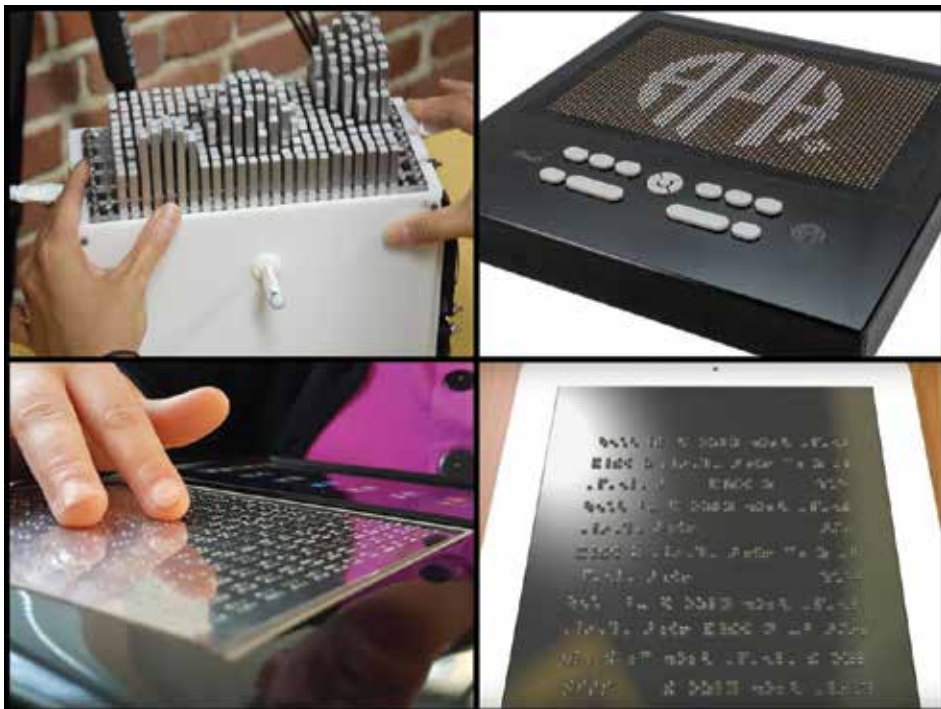
Figure 2. New innovative solutions being developed for individuals with BVI: upper left—demonstration of shapeShift (multi-height pin array) [39]; upper right—Graphiti (refreshable pin array) [37]; lower left—BLITAB (refreshable pin tablet) [38]; and lower right—Holy Braille (microfluidic tablet) [40].
