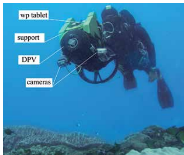
Figure 5. The driver propulsion system (DPV), a remotely operated vehicle (ROV), equipped with a waterproof (wp) tablet and cameras. The tablet is used to coordinate data collection and steer vehicle direction.
