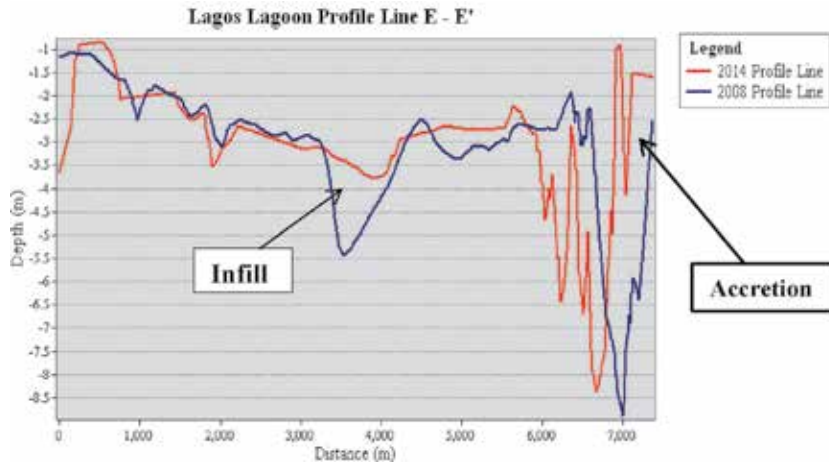
Figure 8. Profile section E-E' showing trend of variation in the repeated bathymetric data.
