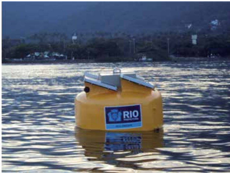
Figure 3. Buoy containing the multiparametric probe multiparamétrica. (Source: Photos supplied by the TECMA, 2016).
