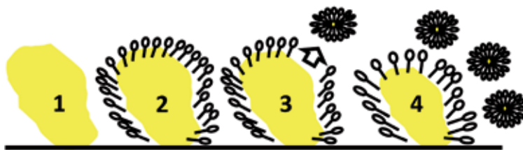
Figure 2. (1) Oily material, (2) adsorption of surfactant on oily material, (3) solubilization of oily material and emulsification, and (4) oily mass removal.
