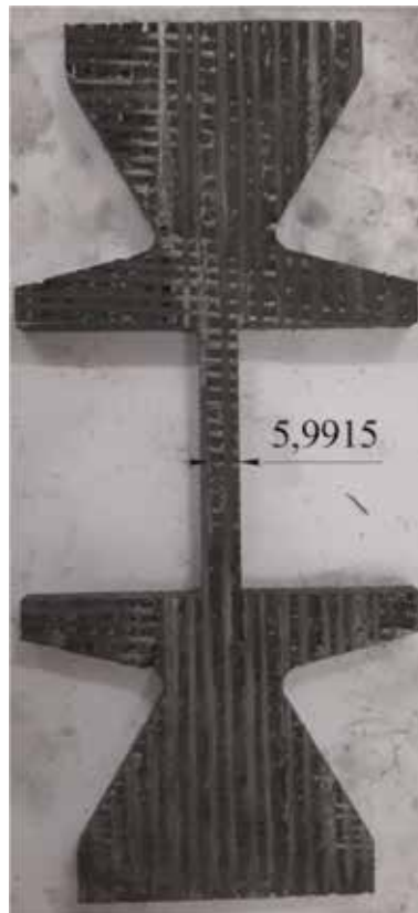
Figure 14. The result of cutting carbon-carbon composites.
