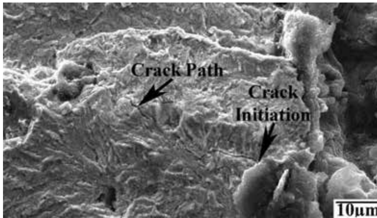
Figure 15. Fatigue fracture at ADI weld metals indicating the crack initiation and crack propagation path.
