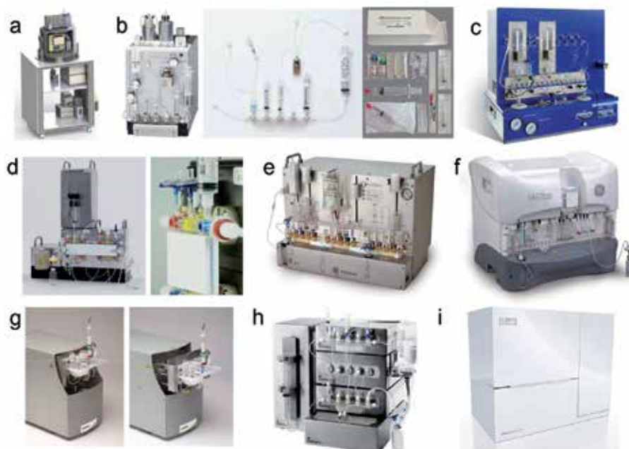
Fig. 2. Commercial cassette-based radiosynthesizers. (a) ABT Biomarker Generator. (b) BIOSCAN F-18 Plus synthesizer (left), disposable cassette (middle), and reagent kit (right). (c) Comecer Taddeo. (d) Eckert & Ziegler PharmTracer. (e) GE TRACERlab MX. (f) GE FASTlab. (g) IBA Synthera in operation (left) and during cassette ejection (right). (h) SCINTOMICS GRP module. (i) Sofie Biosciences ELIXYS.
