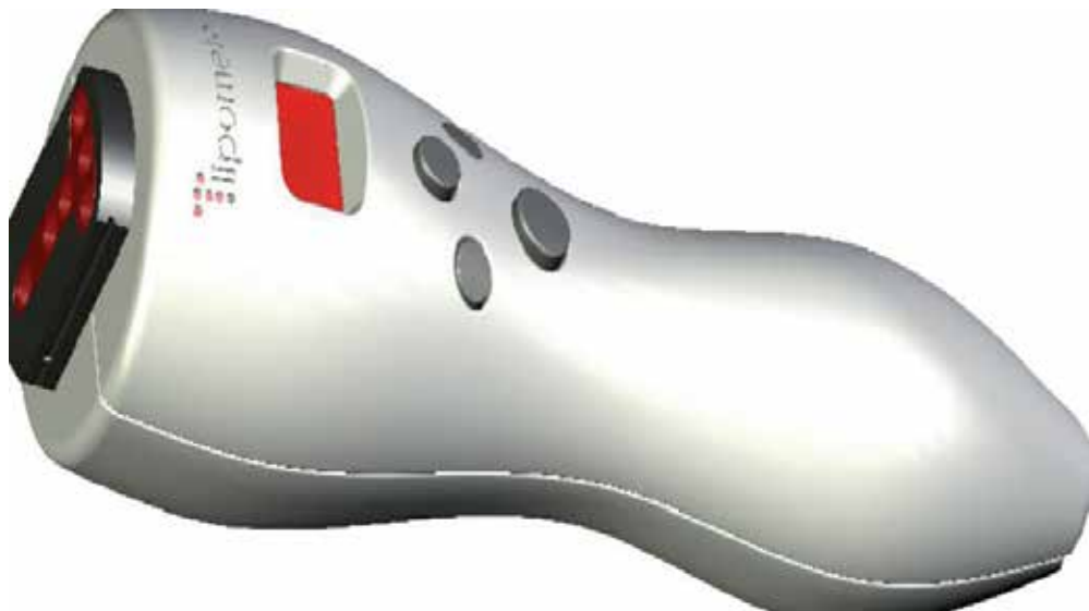
Fig. 1. The Lipometer, an optical device to measure the thickness of subcutaneous adipose tissue layers
