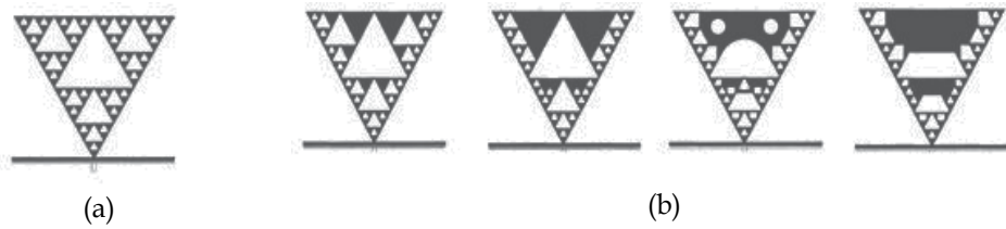
Fig. 32. Printed multiband antenna monopoles a)The self similar ordinary Sierpinski gasket. b) Modified Sierpinski gaskets.
