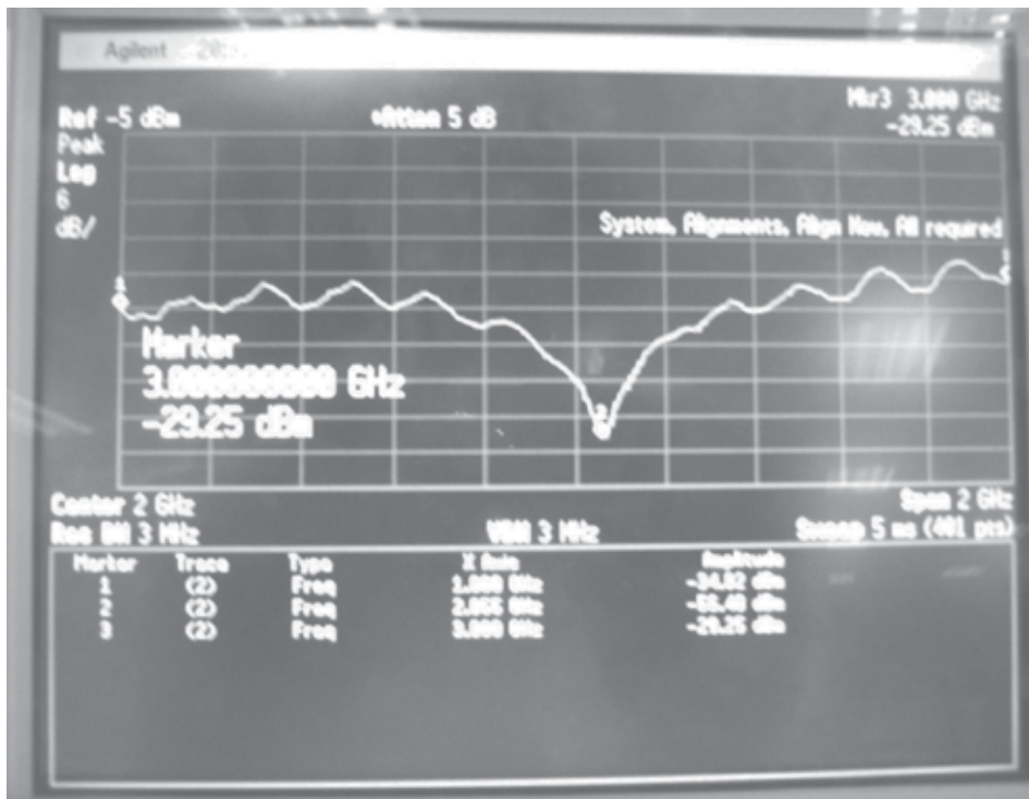
Fig. 16. Measured Power Transmission (1 - 3GHz).
