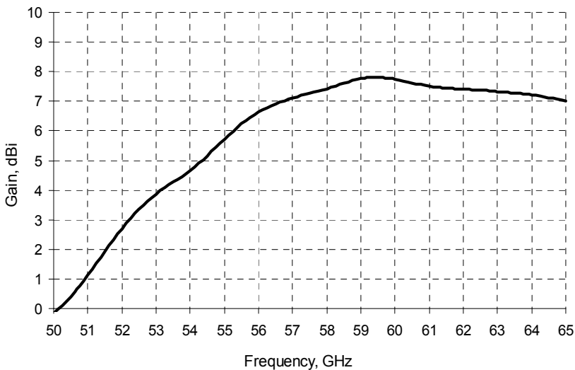
Fig. 3.8. Measured and simulated peak gain versus frequency.
