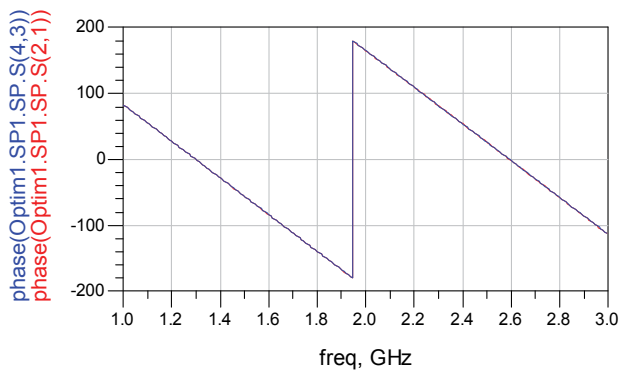
Fig. 17. ADS simulated results for phases of path 2 and reference path
