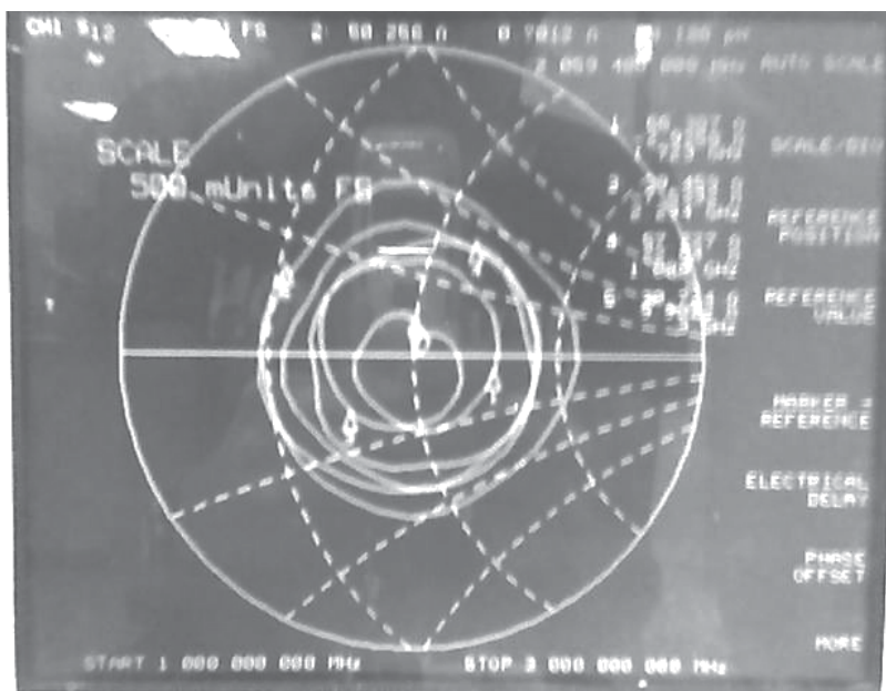
Fig. 18. Measured Impedance Response of Structure.
