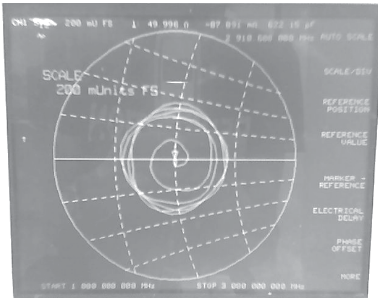
Fig. 8. Measured Input Impedance of DRA Structure.
