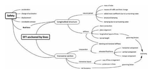
**Figure 15.** *Relation of structural element and safety.*
