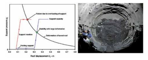
Figure 44. Comparison between rigid (red line) and yielding (blue line) support [18].
