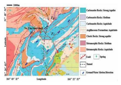
**Figure 3.** Hydrogeological plan of the tunnel area of Yuelongmen tunnel.
