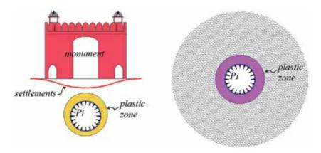
Figure 3. Impact of plastic zone formation around a shallow (left) and a deep (right) tunnel.
