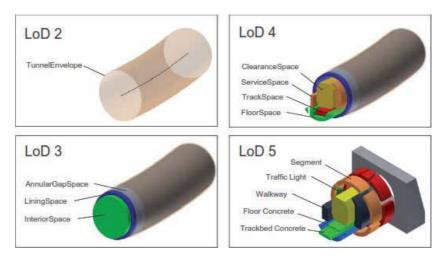
Figure 4. BIM level of development, shield tunnel case [1].
