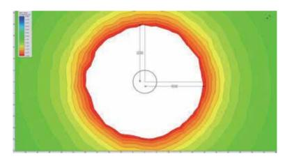
Figure 9. Stress distribution around a circular deep tunnel (Z = 25R, k = 1) [32].
