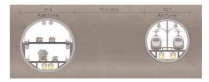
Figure 16. Optimized TBM tunnel alternative. Current cross-section.
