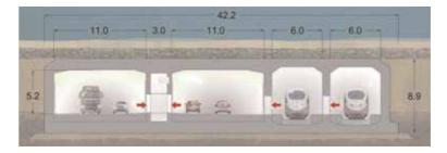
Figure 15. Immersed tunnel solution. Current cross-section.
