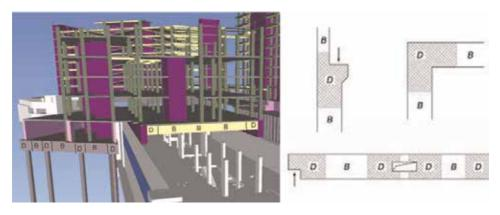
**Figure 10.** *Typical examples of D and B regions in transfer systems.*
