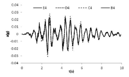
**Figure 10.** The dynamic response of Model 4 with the big tunnel  $(R_2 = 10 m)$  subjected to the Upland excitation.
