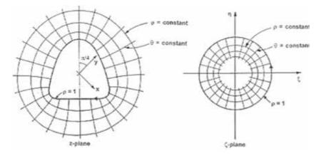
Figure 5. Conformal mapping of an infinite region surrounding a hole onto the unit circle [28].
