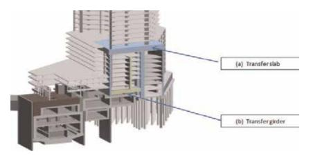
**Figure 6.** *Transfer slab (a) at elevated position and (b) transfer girder.*
