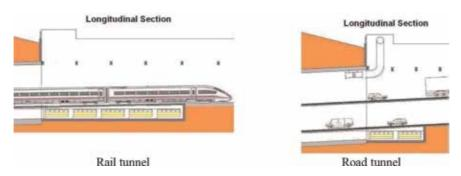
Figure 19. Optimized TBM tunnel alternative. Portals of the tunnels.
