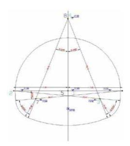
**Figure 3.** *A simplified horseshoe tunnel section.*
