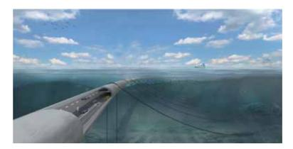
Figure 13. Image of an SFT with positive buoyant tied down to sea bed.
