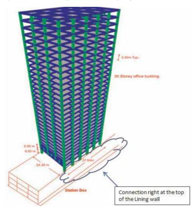
Figure 7. Idealized "module" of TOD "loading" all along the lining walls of the station box.
