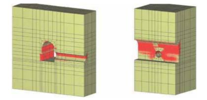
Figure 19. Plastic zone formation around the excavations according to elliptic paraboloid failure criterion [52].
