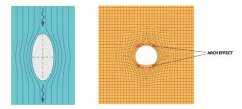
**Figure 2.** Flow lines in the current of a river around a pier (left) and stress field flow lines around a tunnel [1].
