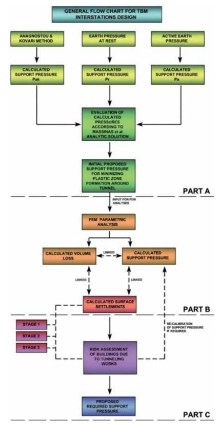
**Figure 14.** Overview of a TBM tunnel interstation design.
