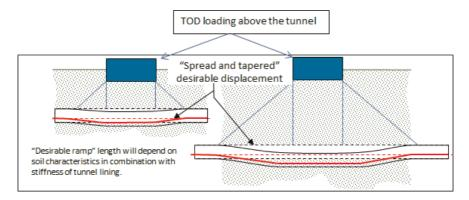
**Figure 19.** *Desired "ramping" of the displacements.*
