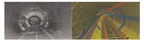
Figure 5. BS-BS laser scan survey and 3D design model.
