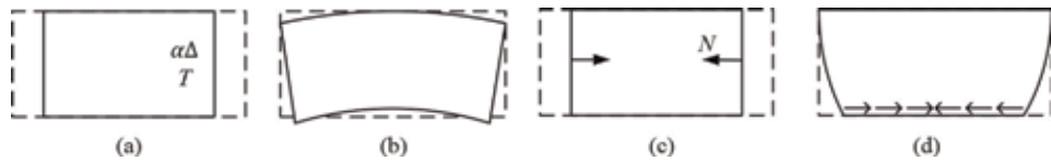
Figure 11. Four components of the deformation in the die or substrate. (a) Longitudinal normal deformation induced by the thermal expansion, (b) longitudinal normal deformation induced by the shear stress, (c) transverse bending deformation, and (d) longitudinal shearing deformation.
