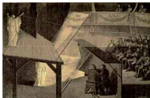
Figure 1. Configuration and projection of the Pepper’s ghost effect on stage.
