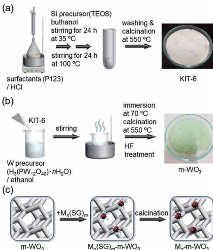
Figure 3. Preparation methods of (a) KIT-6, (b) m-WO 3 , and (c) M n -m-WO 3 (M = Ag, Ni, or Co).
