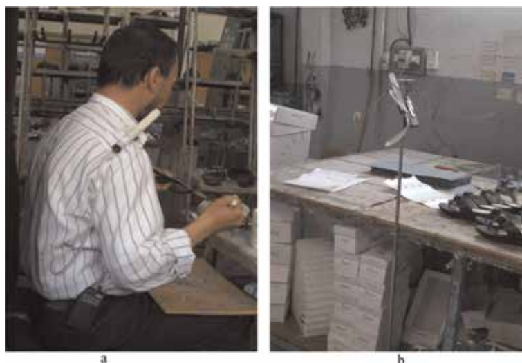
Figure 1 (a) Individual sampling of indoor air exposure. (b) Stationary sampling of the workplace's atmosphere.
