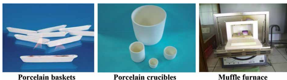
Figure 1. Equipment used in solid-state synthesis.
