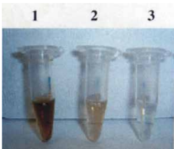
Fig. 2. Visualization of hydrogen sulfide production by precipitation of bismuth trichloride. 1. Poryphyromonas gingivalis ATCC 33277 culture; 2. Subgingival fluid sample ( P. gingivalis positive); 3. Subgingival fluid sample ( P. gingivalis negative)
