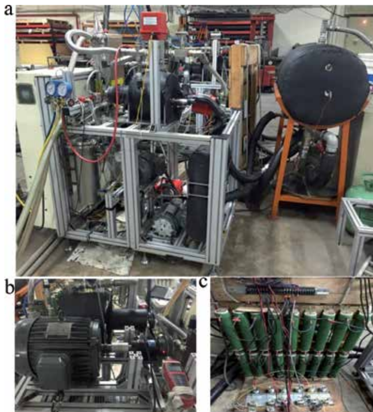
Figure 2. The photos of (a) experimental setup, (b) the expander generator set, and (c) the electrical load.
