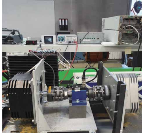
Figure 14. Photo of the test rig – The identical motors are connected in back-to-back configuration.
