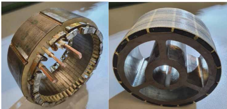
Figure 12. Photo of the prototype. Left: Standalone wound stator with bar winding - Right: Glued magnets on the rotor wheel and sleeved rotor.
