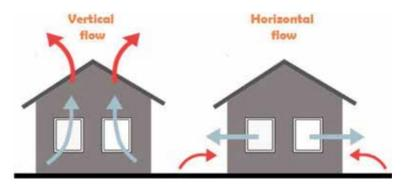
**Figure 2.** Natural ventilation due to difference of temperature.
