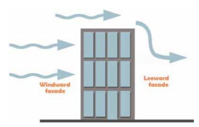
Figure 1. Natural ventilation due to difference of pressure.
