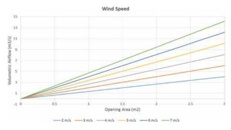
Figure 6. Volumetric airflow by varying the wind speed and the effective opening area.
