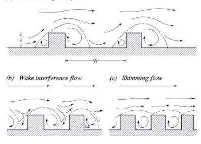
Figure 7. The different flow regimes in urban canyons over building arrays of increasing H/W ratios [1].
