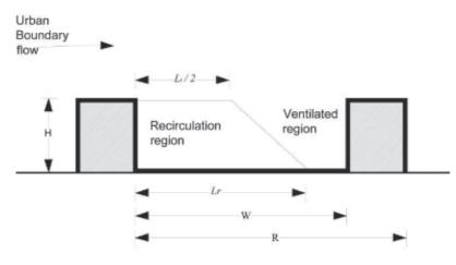
Figure 6. Cross section of a street canyon showing the dimensions of the regions.
