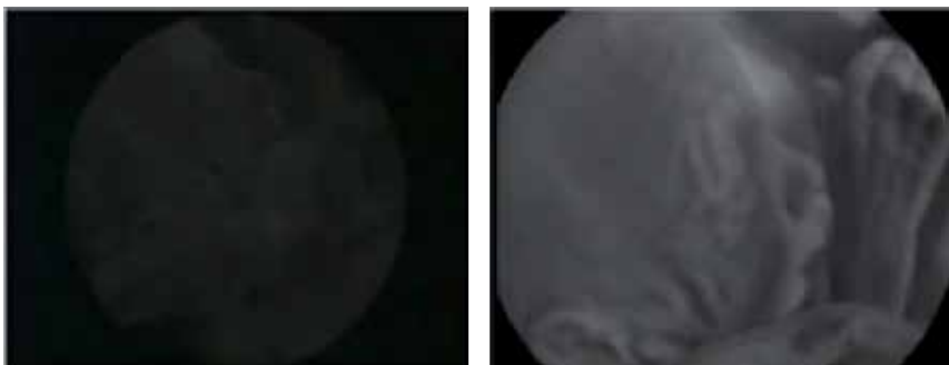
Fig. 4. Comparison of endoscopic image of an intrauterine fetal phantom model without conventional light source. Left: Conventional endoscopic image. Right: New ultra-high sensitive endoscopic image.
