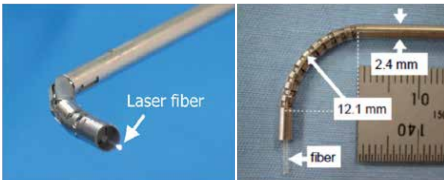
Fig. 7. Distal-end part of the miniature bending laser manipulators with a laser fiber. Left: Wire-guided linkage-driven 3.5-mm manipulator. Right: Wire-driven 2.4-mm manipulator.
