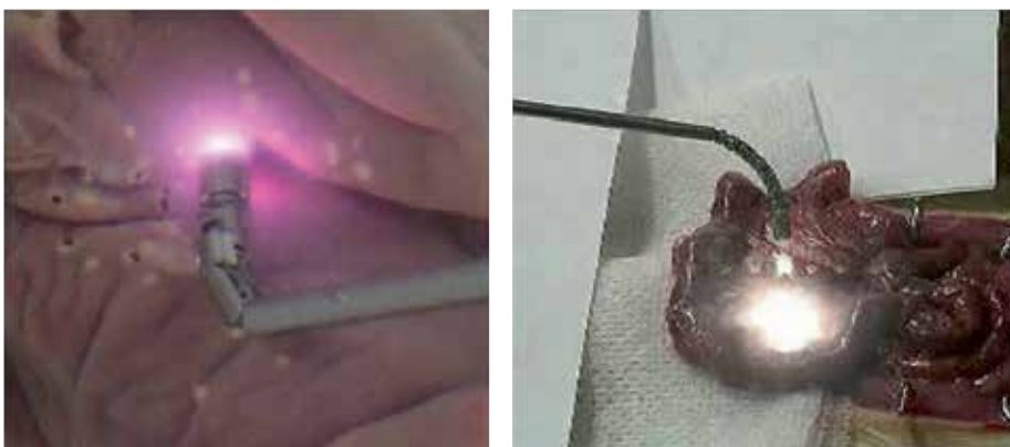
Fig. 8. Left: Nd:YAG laser photocoagulations of the placental phantom model surface with bending motion of the 3.5-mm laser manipulator. Right: Nd:YAG laser photocoagulation of the vessels on the rat mesenterium with the wire-driven 2.4-mm bending laser manipulator.
