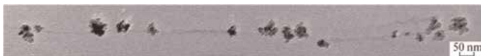
Figure 1. Initial stage of curing of the epoxy matrix in the presence of COOH-functionalized CNTs. Reprinted with permission from IAPC “Nauka” [39].
