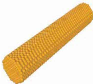
Figure 1. Structure of rod-shaped Au nanoparticle generated by lamps ( D = 6.3 nm, Lz = 61.86 nm, D:lz = 0.1 , and 111147 atoms). The atomic structures are visualized by Ovito.
