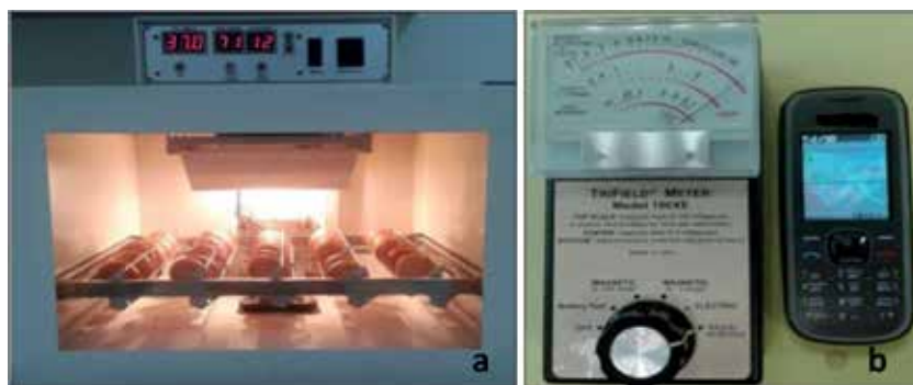
Figure 2. (a) The egg incubator. (b) TriField meter showing high levels of electromagnetic waves transmitted from the mobile during call receiving ( \geq 1 mW/cm 2 ).
