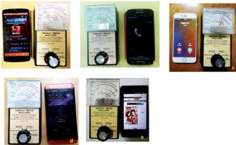
Figure 1. TriField meter measuring the electromagnetic field exposure when the phone is receiving a call (the needle moving toward the right with increasing intensity of the electromagnetic waves) (a) group 1, (b) group 2, (c) group 3, (d) group 4, and (e) during downloading, the needle is hitting extreme right.
