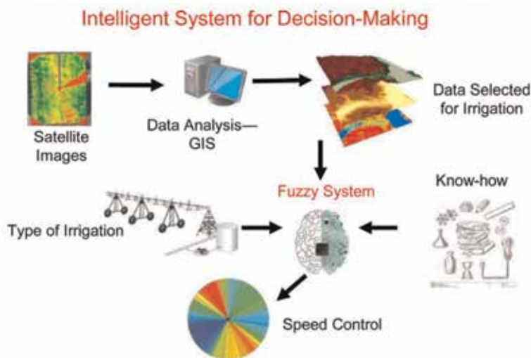
Figure 7. Structure for intelligent irrigation system strategy.
