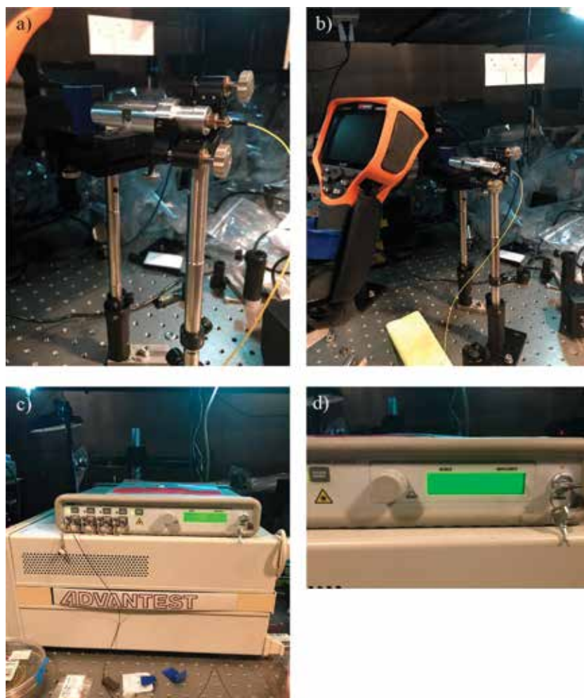
Figure 6. Images of the installation of the (a) 820 nm wavelength laser, (b) non-contact digital IR thermometer, (c) connection to the multi-channel laser source, and (d) selection of the channel with the desired wavelength.
