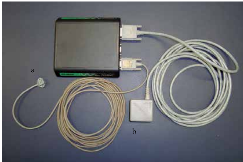
Fig. 1. Illustration of the Polhemus system. a) sensor coil; b) transmitting coil.
