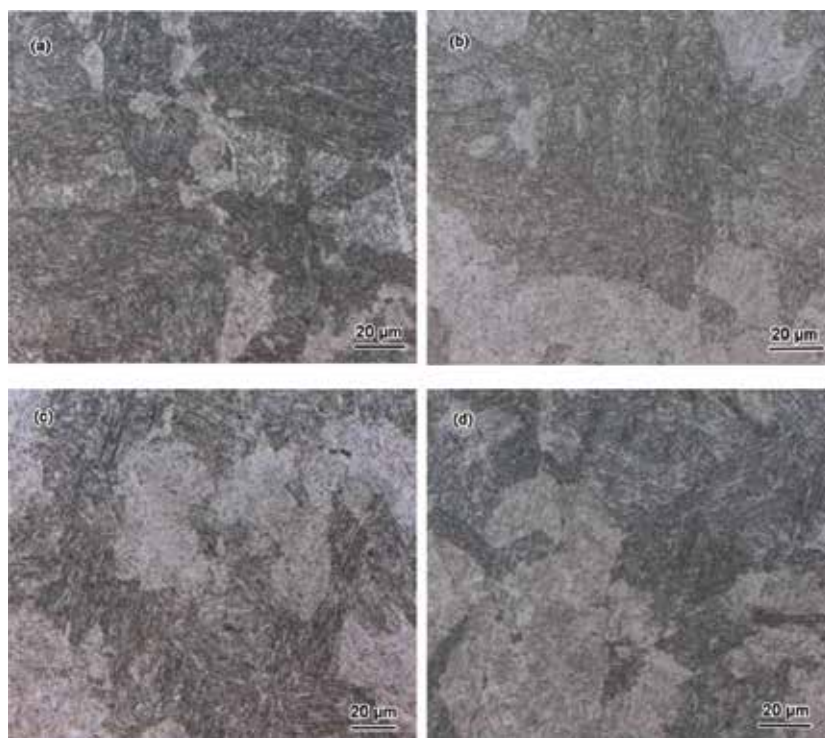
Figure 13. OM images of specimen Case I under different cooling rates. (a) 0.02°C/s; (b) 0.2°C/s; (c) 0.5°C/s; (d) 1°C/s.
