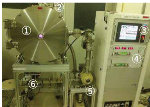
Figure 1. RF-DC plasma nitriding system. (1) Vacuum chamber, (2) RF-generator, (3) control-panel, (4) RF- and DC-power suppliers, (5) evacuation units, and (6) carrier gas supply.
