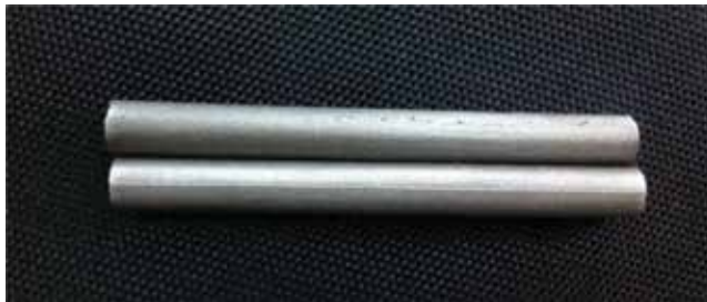
Figure 1. Specimens for the free dilatometry test.
