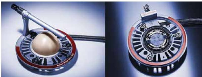
Figure 4. Oven coupled to the X-ray diffractometer.
