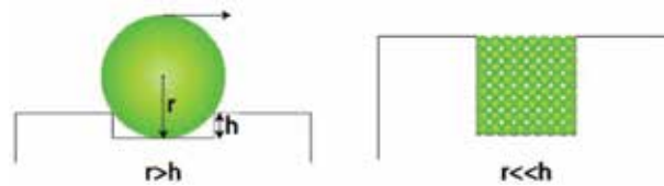
Figure 12. The effect of relative size of surface texture and additive particles: particle with similar dimensions as the profile and particles smaller than the valleys of the texture [63].
