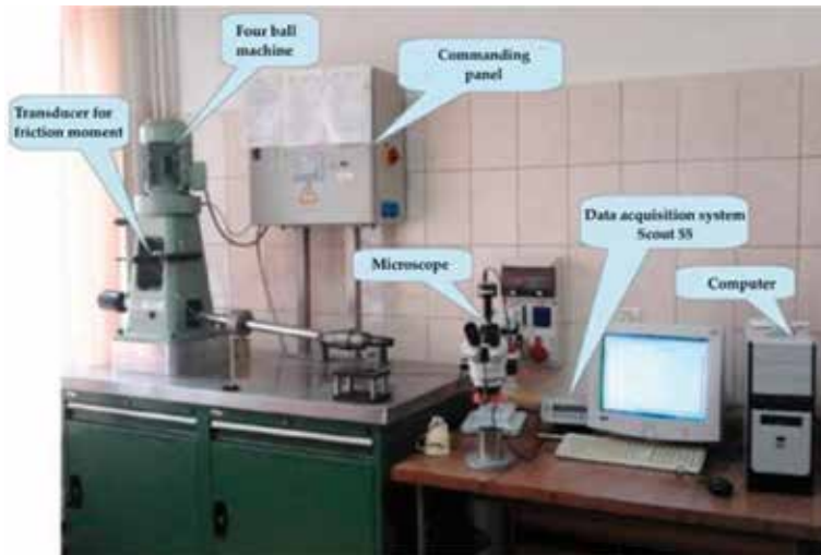
Figure 14. Four ball machine ("Lubritest" Laboratory, "Dunarea de Jos" University of Galati).
