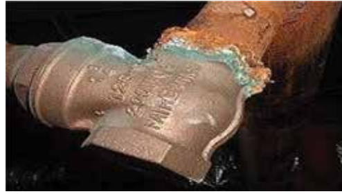
Figure 3. Schematic representation of galvanic corrosion.
