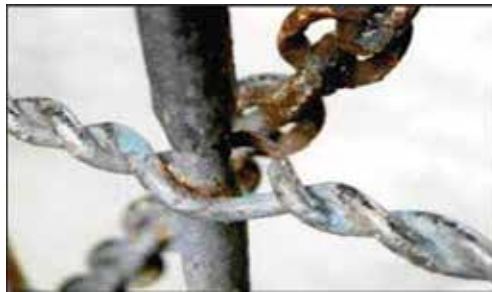
Figure 10. Schematic representation of fretting corrosion.
