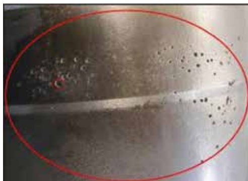
Figure 11. Schematic representation of cavitation corrosion.
