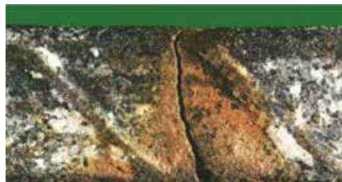
Figure 9. Schematic representation of stress corrosion.
