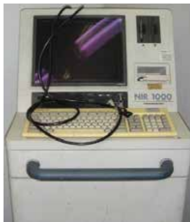
Figure 4. The NIRO 1000 (Hamamatsu Photonics K.K., Japan) used in the first functional near-infrared spectroscopy experiment [7–9].
