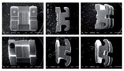
Fig. 1. Top line: Scanning electron microscopy of one bracket of standard edgewise appliance from a frontal (A), lateral (B), and oblique (C) view. Bottom line: Scanning electron microscopy of one straight wire bracket from a frontal (D), lateral (E), and oblique (F) view. The absence of information in the slot of the bracket of standard edgewise appliance in comparison with the bracket of the straight-wire appliance can be observed.
