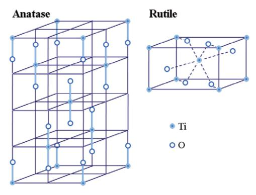
Fig. 3. Anatase and rutile forms of crystalline TiO<sub>2</sub>.
