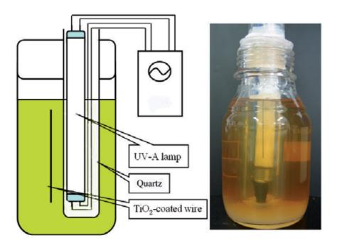
Fig. 2. Apparatus for the assay of anti-adhesion effect of TiO<sub>2</sub>-coated orthodontic wire.
