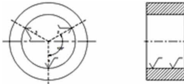
Figure A3. Three radial locations each at 120° in one plane and to be measured in three planes for bearing (total 9 readings).
