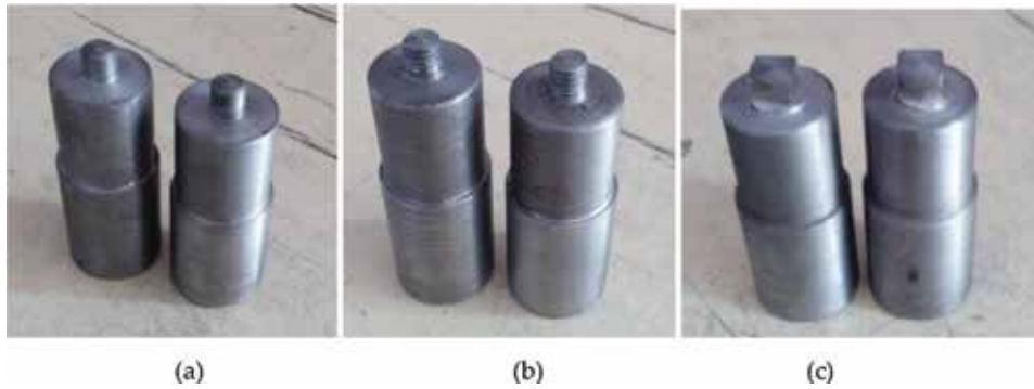
Figure 3. FSW tools (a) straight cylindrical pin, (b) threaded straight cylindrical pin, (c) square pin.
