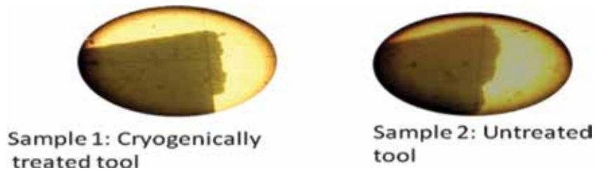
Figure 4. Wear measurement of the specimens using a toolmakers microscope.
