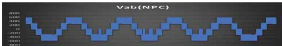
Figure 8. Output voltage of NPC Inverter.
