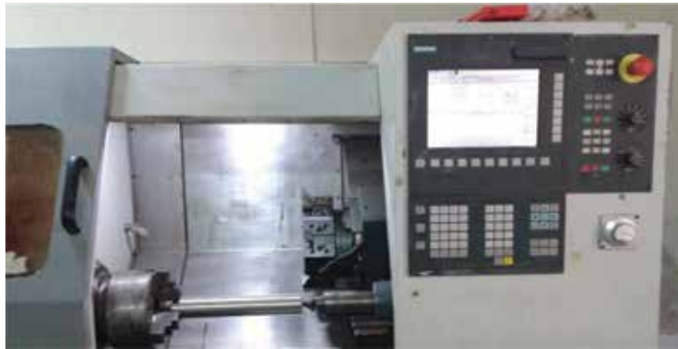
Figure 1. CNC turning centre STC-200.
