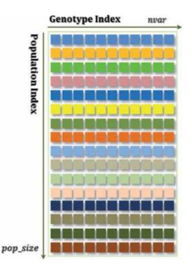
Figure 5. 2D view of the chromosome-based layout in global memory.
