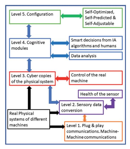
Figure 1. Cyber-physical architecture that includes five levels.
