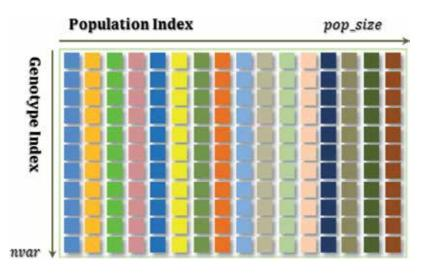
Figure 6. 2D view of the genotype-based layout in global memory.
