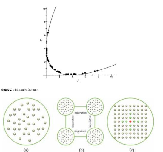
Figure 3. Models of parallel GAs. (a) Master-Slave model, (b) Island model, and (c) Cellular model.
