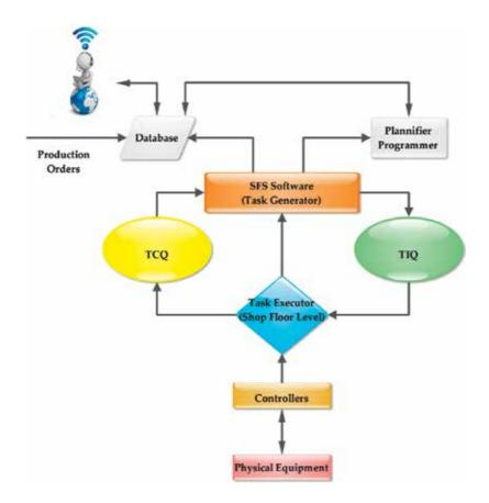
Figure 1. SFS based production control architecture in Industry 4.0. ([16] p. 382, 2005).
