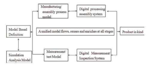
Figure 2. Principle of digital thread.
