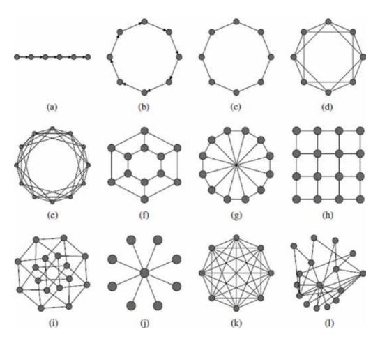
**Figure 8.** Common migration topologies (from [16]). (a) Chain, (b) I-way ring, (c) Ring, (d) +1+2 ring, (e) +1+2+3 ring, (f) Tours, (g) Cartwheel, (h) Lattice, (i) Hypercube, (j) Broadcast, (k) Fully-connected, and (l) Barabasi-Albert (3.2).
