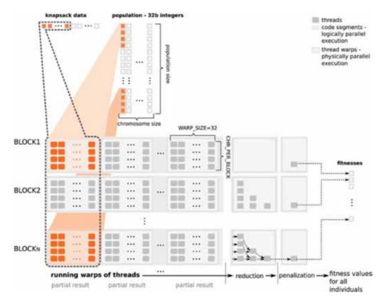
Figure 9. The configuration of kernel execution (from [17]).
