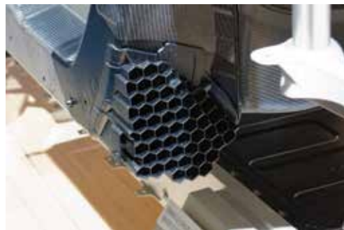
Figure 1. The use of stacked-joined hexagonal lightweight pipes for a car bumper [6].
