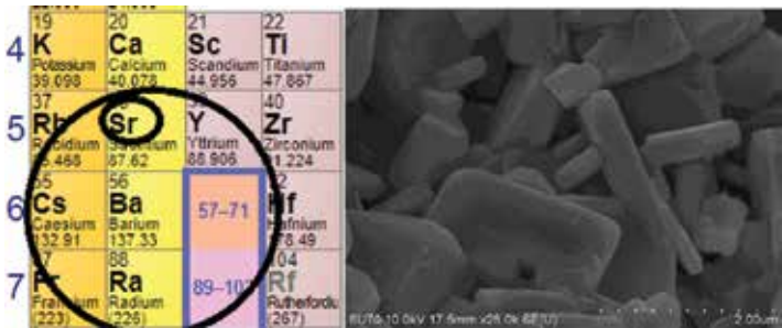
Figure 8. SEM micrograph of (\text{Ba}_{0.95}\text{Sr}_{0.05})\text{TiO}_3 with microstructure cubic grain.
