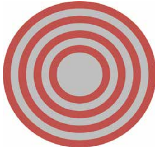
Figure 2. Cross-sectional view of a typical omniguiding Bragg fiber comprised of periodic multi-layered dielectric mirrors.
