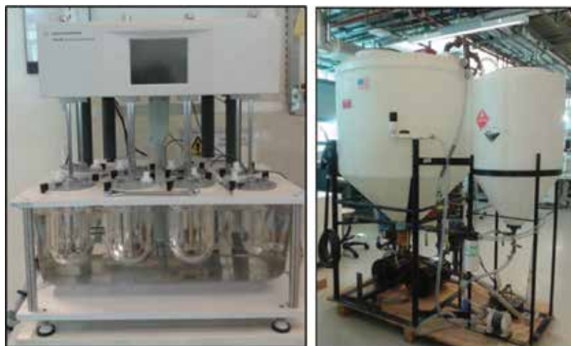
Figure 1. Dissolution apparatus representing eight multiple 1-L batch reactors and HomeBiodieselKits 500-liter batch reactor.
