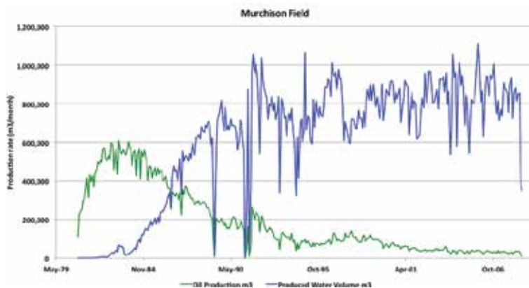
Figure 2. Oil and water production profile for the Murchison field, North Sea.
