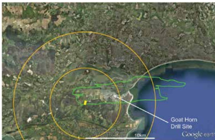
Figure 5. Location of the Wytch farm oilfield (outline in green) relative to the Poole and Bournemouth (top right hand corner of figure) urban areas. The concentric circles are 5 and 10 km radius and centred on the Wytch farm gathering station. District heating schemes typically lose up to about 1°C km -1 of insulated pipe [8]. GH is the location of the Goathorn peninsula from where long reach, horizontal wells were drilled into Poole harbour and is the location of the well heads closest to Poole-Bournemouth [9]. Base image from Google earth.
