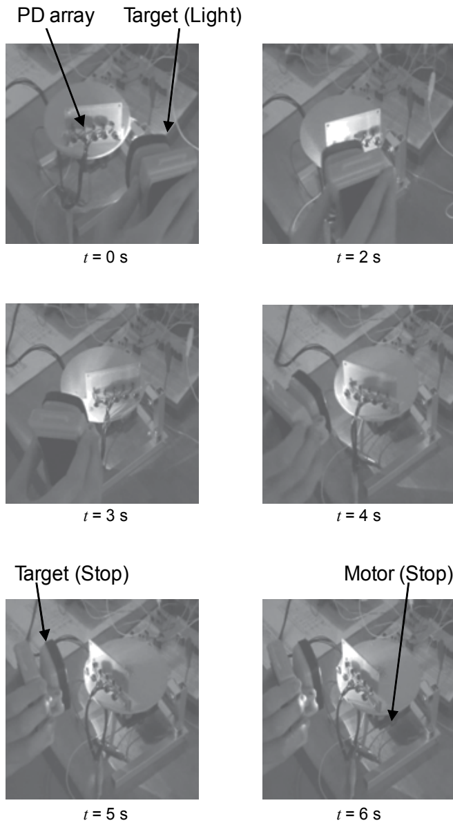
Fig. 7. Measured results of the test system when the target moves toward the left side.
