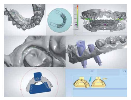
Figure 11. Processing of intraoral scan data for model building.
