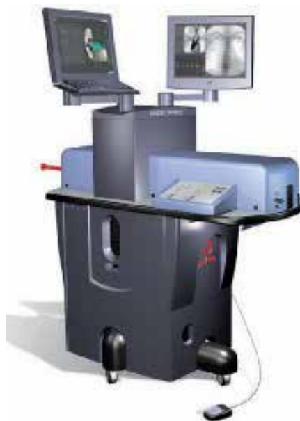
Fig. 2. ANGIO Mentor endovascular surgical training simulator
