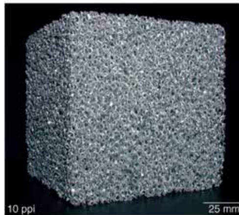
Figure 2. A piece of FeCrAlY foam sample manufactured with the sintering route [22].
