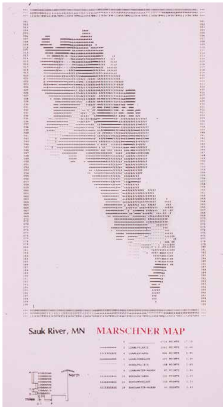
Figure 2. A map of the Sauk River, Minnesota pre-settlement vegetation. Back in the mid-1980s, black and white alphanumeric GIS maps were often the standard. The technology had been transferred down from mainframe computers to the recently developed micro-computers (copyright 1983 Jon Bryan Burley, all rights reserved, used by Permission).
