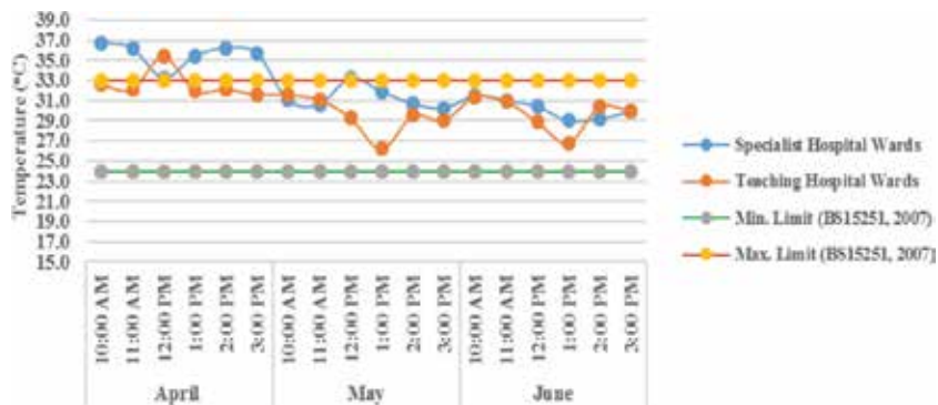
Figure 18. Monthly temperature variation in the hospital ward buildings.
