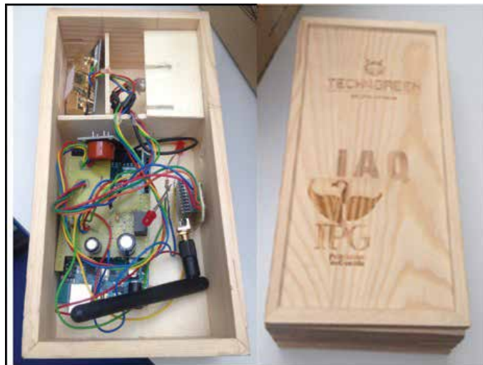
Figure 2. iAQ Sensor hardware, from [29].
