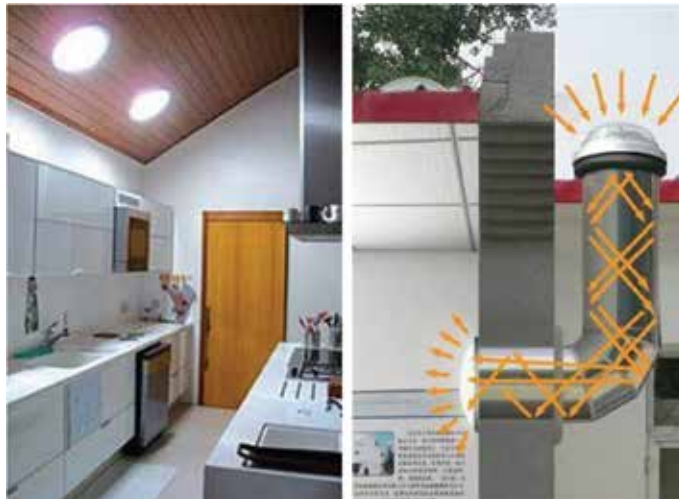
Figure 9. Solar light pipes system. Source: Google Search—Images.
