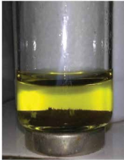
Figure 2. Image of simplified recovery technique of spent magnetic material after adsorption of precious metals [3].
