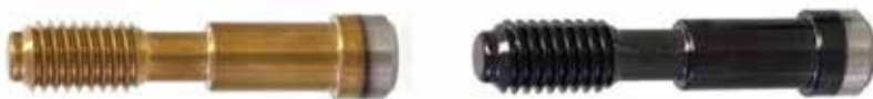
Figure 6. TiN magnetron sputtering coating (left) and diamond-like carbon (DLC) magnetron sputtering coating (right) on Ti dental implant. Courtesy of the commercial company Flubetech.
