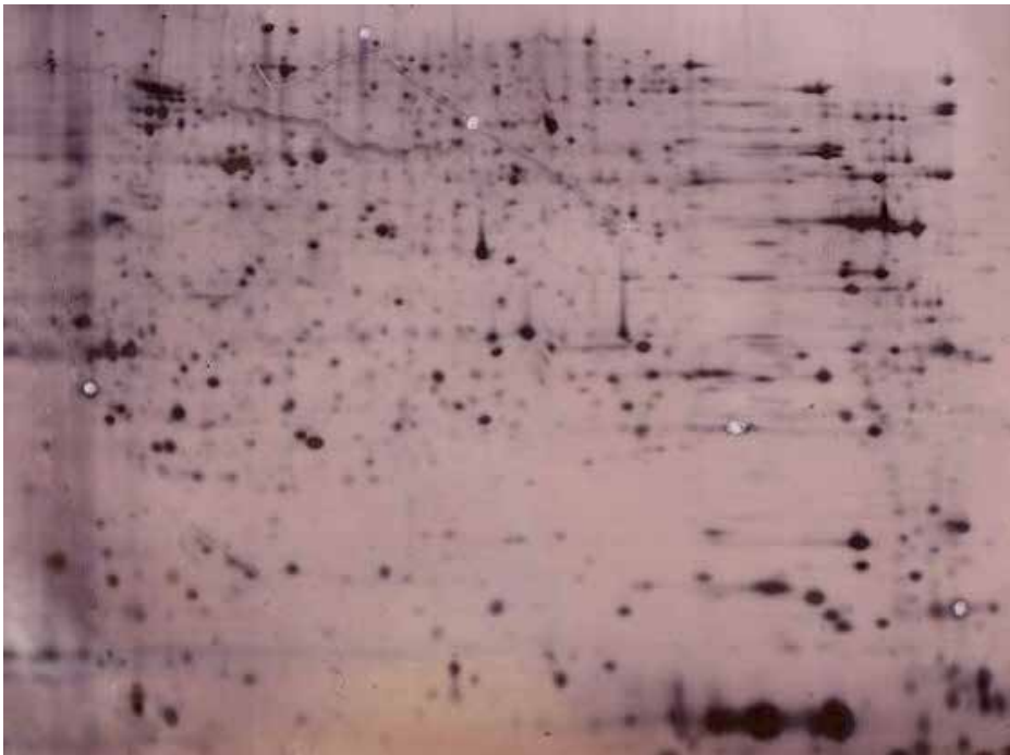
Fig. 2. Silver staining of acrylamide gel after SDS-electrophoresis Protein extract (600 µg) from cerebellum was loaded in a first dimension IPG strip (pH3-11, NL, 24 cm; Running time: 15.5 hr, approx 47 kVh) and resolved in 12.5% acrylamide gel (Running time: 5.15 hr, 10 W per gel). Proteins were visualized by silver staining. These gels are called preparative gels, and they contain more protein content to allow for subsequent analyses including silver staining and MALDI-TOF. CyDye labelled proteins were run on analytical gels which are scanned by lasers and thus do not require a high quantity of proteins.
