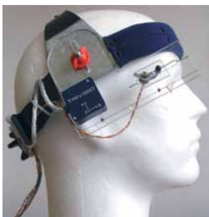
Fig. 5. Combined inertial system with infrared marker for detecting the position by IR camera system.
