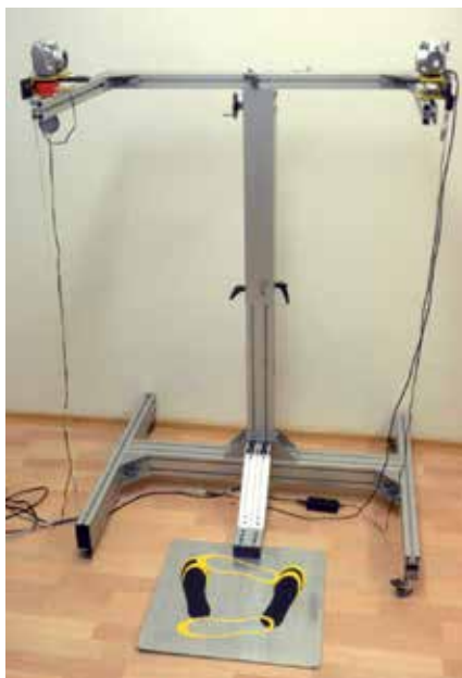
Fig. 4. The two-arm stand with fixed two cameras and laser collimators designed for the precise adjustment of the system.
