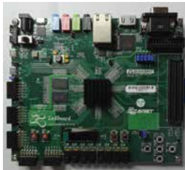
Figure 11. Zedboard development board used for two of the UKF implementations.
