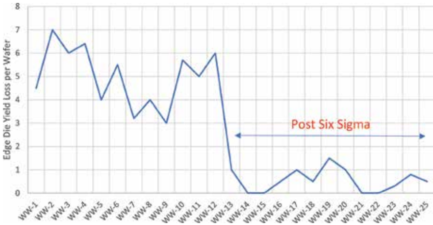
Figure 14. Edge die yield loss graph over 26-week time frame.
